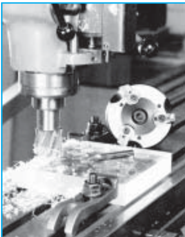
Fig. 24: Routing of PLEXIGLAS® with shell endmill; various other cutter types: (a) double-fluted cutter; (b) cylindrical cutter; (c) diamond cutter
