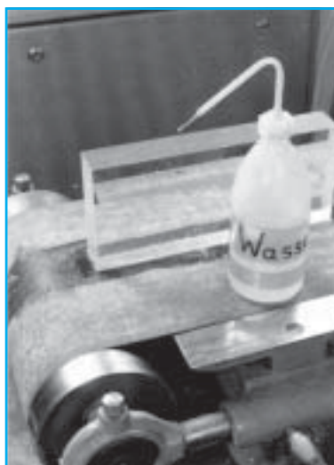
Fig. 38: Wet sanding on a belt sanding machine
