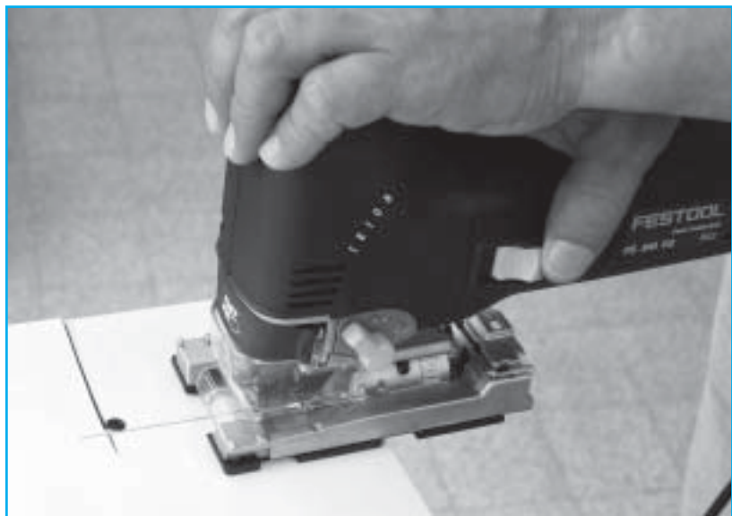
Fig. 10: Jigsawing after predrilling
