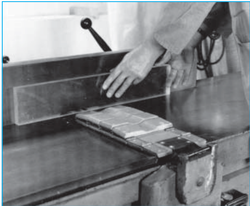
Fig. 36: Smoothing the edges with a surface planer
