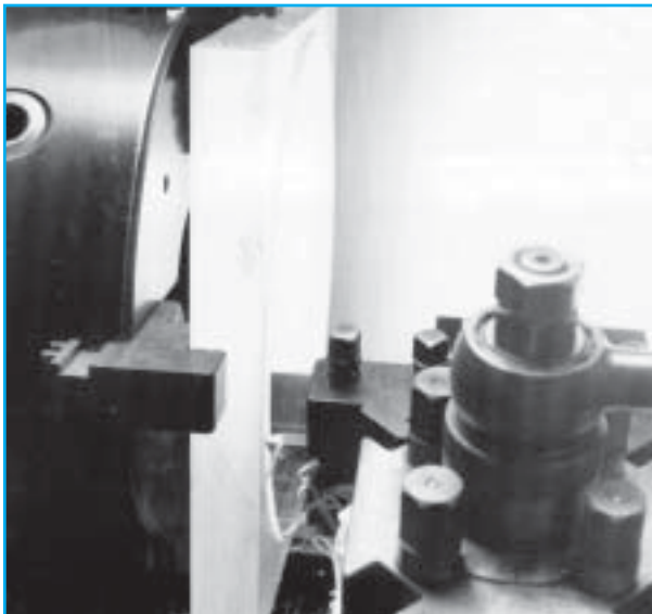
Fig. 31: Turning off a block of PLEXIGLAS® GS
